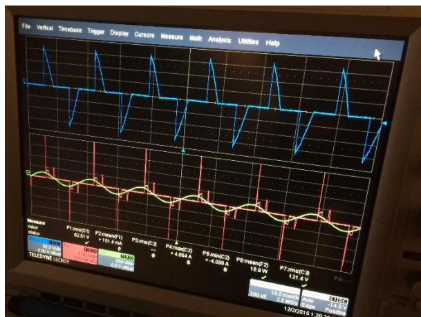
Figure 2: measuring repetitive inrush currents. Source: Lutron Electronics, Coopersburg, USA.
