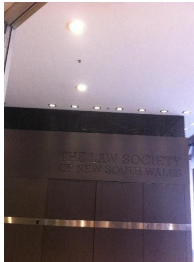
Figure 1: Sign suffering from poorly implemented lighting energy efficiency upgrade. For reference, the sign is barely visible just below the dark band at the top of the wall.
