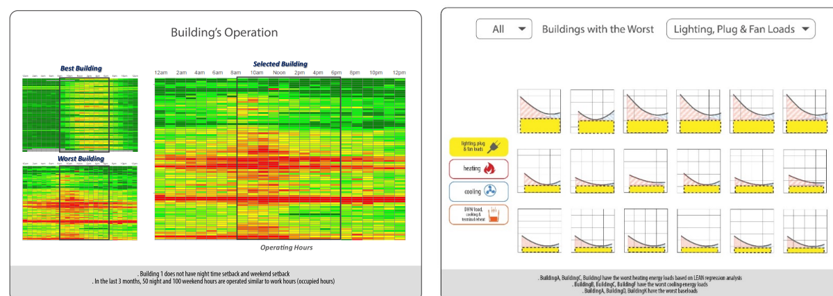
Figure 8: This “heat map” graphic on the left provides an hourly overview of the building energy usage and the LEAN regression data graphic on the right isolates heating, cooling and baseload energy consumptions.
