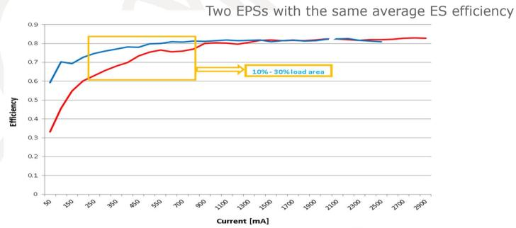
Even if the Energy Star calculation of the average energy efficiencies (mean of the efficiencies at 25%, 50%, 75% and 100% of the rated load) gives very similar results, the differences in the efficiency behavior are often clearly noticeable.
