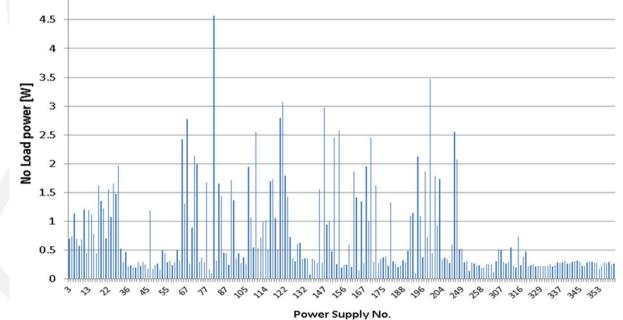
The range of efficiency is quite wide. Many very good (low) values below 0.1–0.15 W, but very inefficient equipment (even higher than 2W) are frequent too. Mobile charger have shown it is possible to have even better efficiency (< 30 mW).
